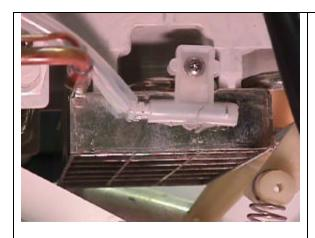
The freeze cycle is controlled by a thermistor, which is mounted at the evaporator outlet. The pump is spraying water up into the evaporator cells to form the square IM cubes. The evaporator temperature lowers as the ice cubes form.
